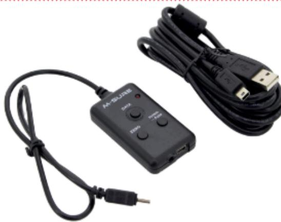
The M-SURE T1 data USB interface features a status LED that flashes to indicate the measurement device is connected. Pressing the DATA button on the interface will paste the displayed information directly into any Microsoft Windows-based software such as Excel. Wherever you position the cursor the displayed value will be inserted. There is also a carriage return to skip to the next line/cell in preparation for the next value.
